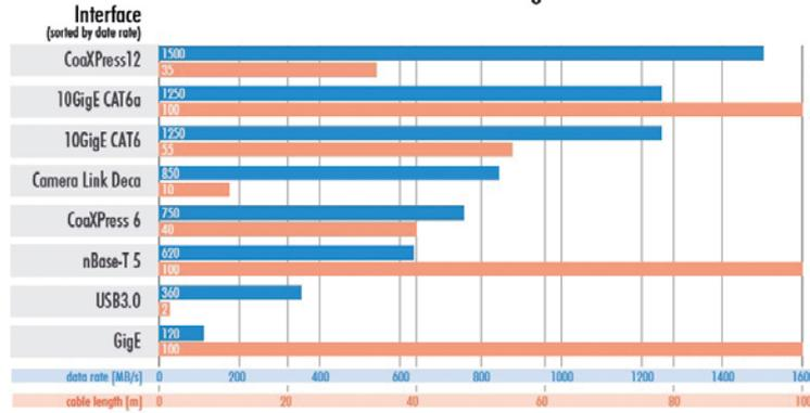
With a maximum transmission speed of around 1250 MB/s, 10 GigE Vision ranks between Camera Link and CoaXPress.
