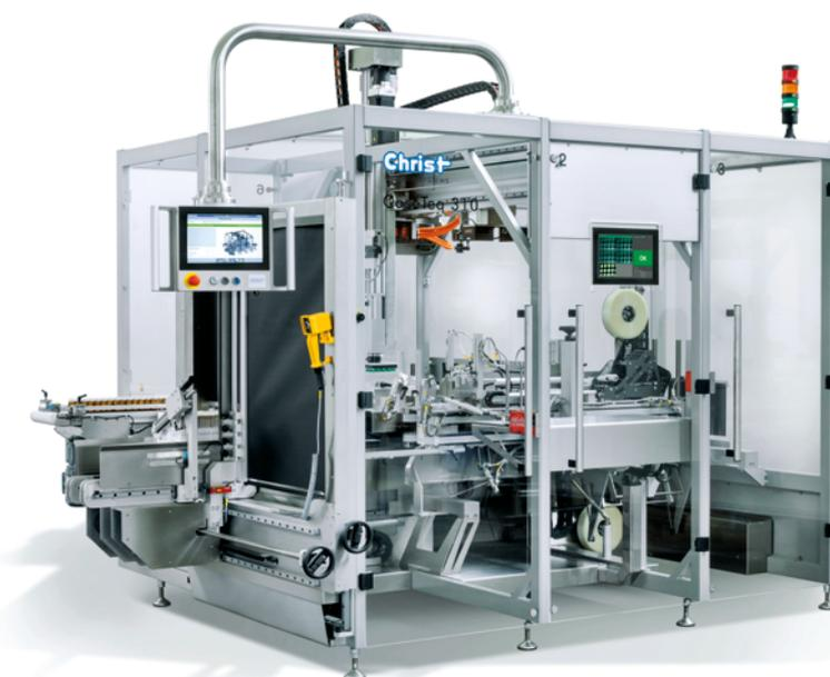
The Caseteq case packer from Christ is a fully automatic horizontal system for erecting, packing and closing pre-glued shipping cases. Cameras from B&R will now be performing various inspection tasks.
