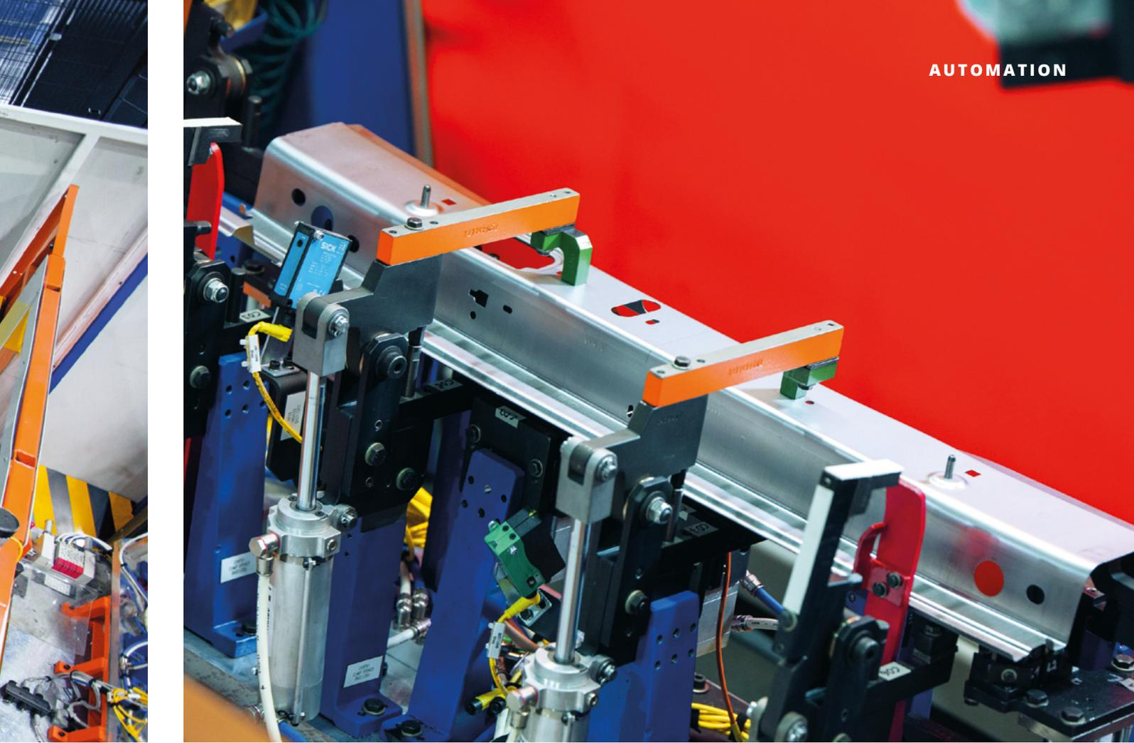
Various stamped and deep-drawn metal sheets are welded to form a supporting element of the bodywork.
