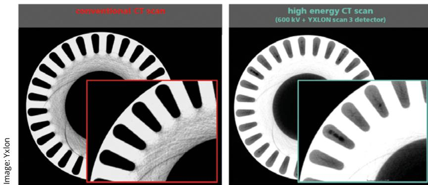
Conventional CT scan of a cast rotor with insufficient resolution of the rotor conductor bars (left) and CT scan with Yxlon FF85 CT system, 600 kV and CTScan 3, showing axially continuous cavities in the rotor conductor bars (right)
