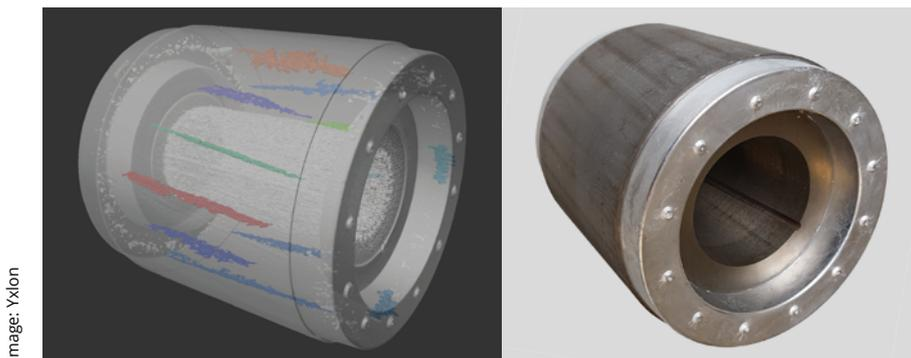
Three-dimensional representation of the casting defects and defect distribution from the high-resolution CT (left) and photo of the cast rotor which externally appears free from defects (right)
