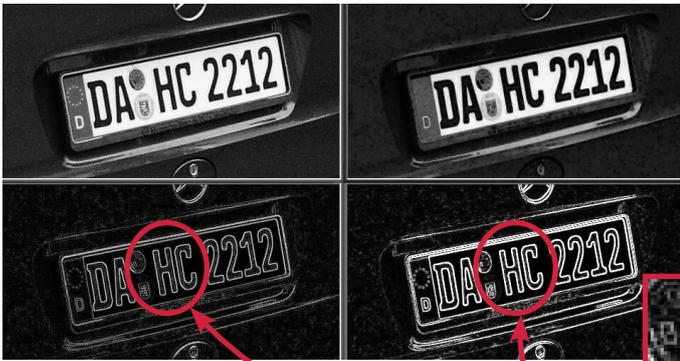
Fig. 2: Grey level image, dilated grey level image (upper part) and the difference of these images (lower left part); in the right left part the result of a Sobel filter for comparison, with enlarged detail from the edge images
