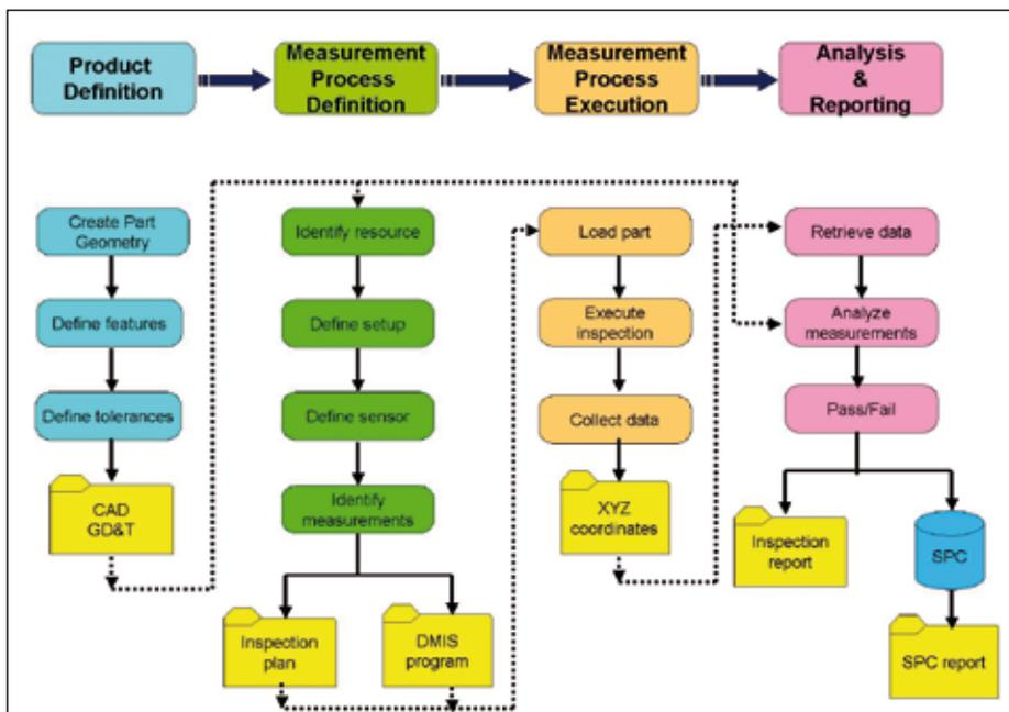
Fig. 1: Traditional CMM-based inspection workflow diagram
