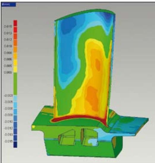
Fig. 3: Deviation colour map of a turbine blade
