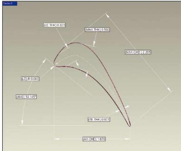
**Fig. 5: 2D sectioning and dimensioning**
