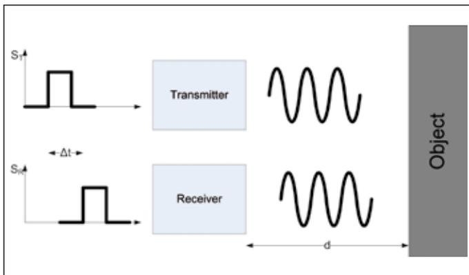
Fig. 3: Pulsed TOF measurement principle
