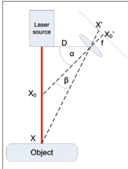
Fig. 2: Triangulation principle
