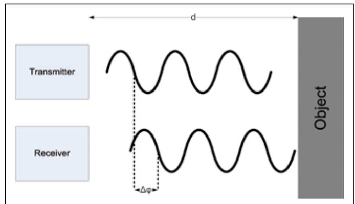
Fig. 4: Modulated Continuous Wave TOF measurement principle
