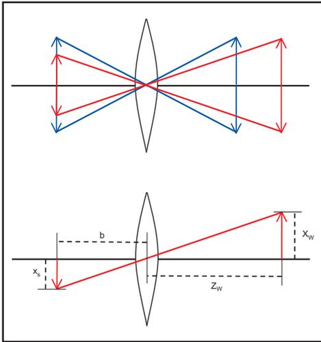
Fig. 2: Central projection in the pinhole-camera model
