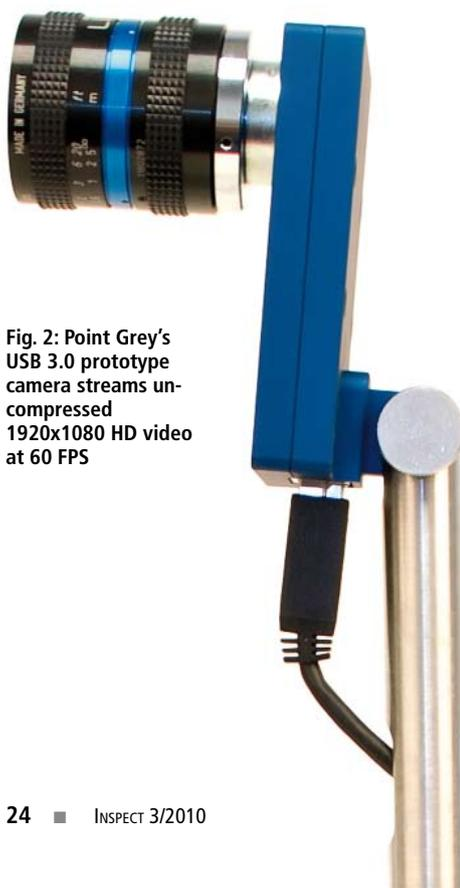
Fig. 2: Point Grey's USB 3.0 prototype camera streams uncompressed 1920x1080 HD video at 60 FPS
