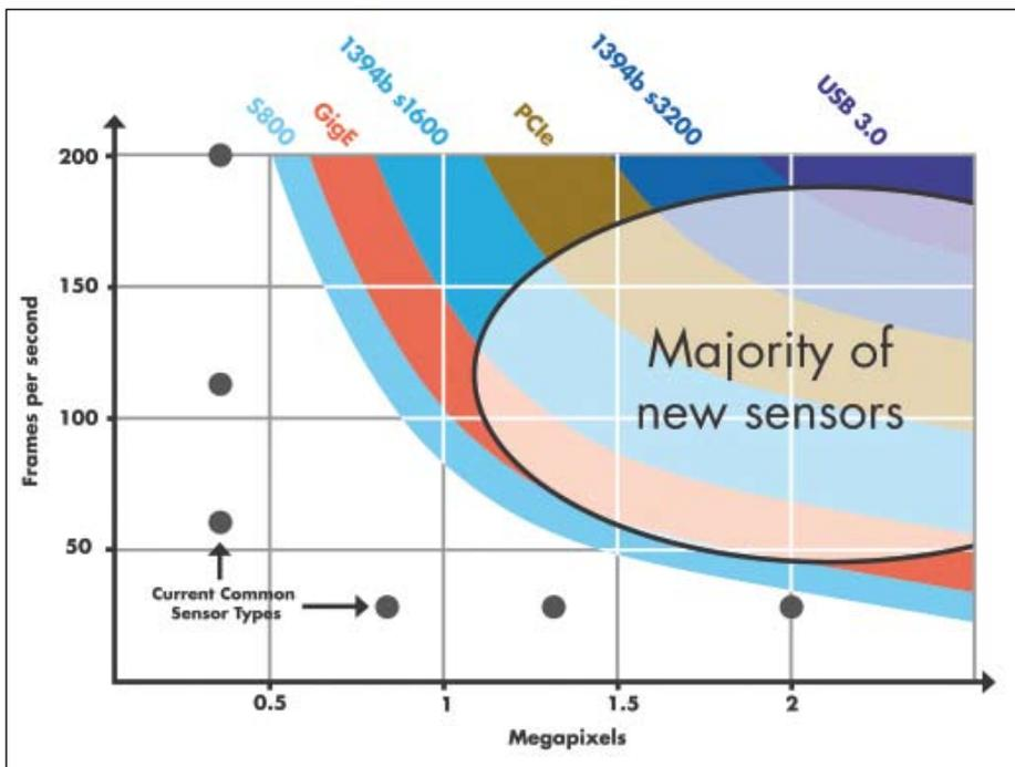
Fig. 4: Most existing digital interfaces do not provide the required bandwidth for many new image sensors
