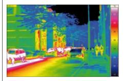
ahead until it is nearly too late. In such situations infrared cameras could provide a better level of safety. Objects at roughly body temperature are luminous in the infrared region at a wavelength of around 10  $\mu$ m. Detectors in the camera register this thermal radiation and locate the source of heat.
