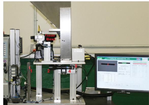
Figure 2. Formed pins in a feeder bowl, are serialized and dropped past a collimated light (1) and photosensor. A part image is taken through a telecentric lens (2) with a high-speed camera (3). The Teledyne DALSA Vision Appliance (4) processes the image to gauge the pin part. The operator interface is shown on the right.
