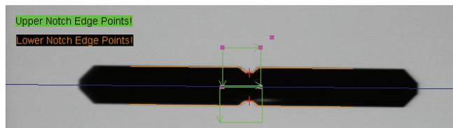
Figure 1. A pin part as seen "in flight" and measured by Teledyne DALSA's Sherlock software.
