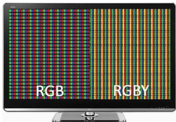
**Figure 6** - Adding a yellow filter to the traditional red-green-blue display yields a brighter, more colorful picture at the cost of reduced sub-pixel size.
