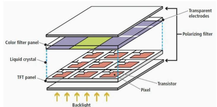
**Figure 2 - A color liquid crystal display typically has the color filter on one of two panels encapsulating liquid crystal material.**
