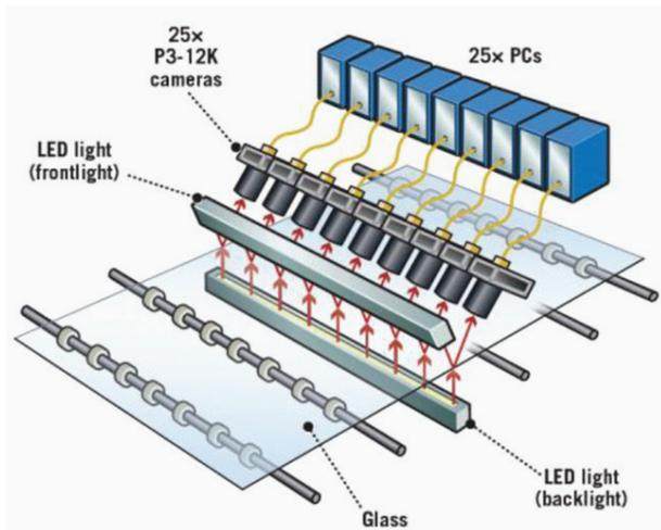
**Figure 5** - LED illumination from both the front and back sides of the panel under inspection allows the Cobra system's cameras to detect a wide variety of defects in the glass and filter array.
