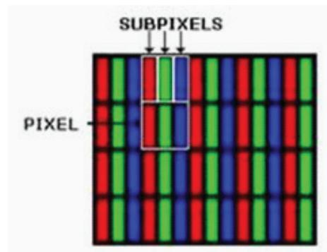
**Figure 1 - Flat panel display pixels comprise three sub-pixels in primary colors.**
