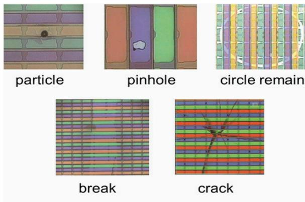
**Figure 3** - Inspection can identify and determine the position of both repairable and non-repairable defects.
