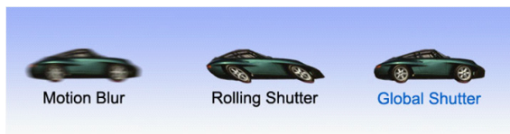
Figure 3: Global shutter, rolling shutter and image distortion
