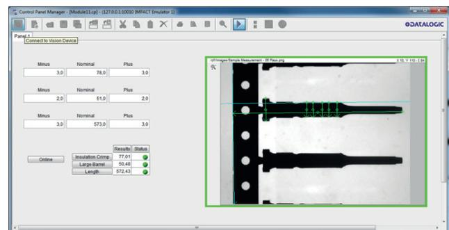
Example for the user interface of a system to inspect metal anchor bolts, which has been created and linked to the image processing algorithm by Graphical Programming
