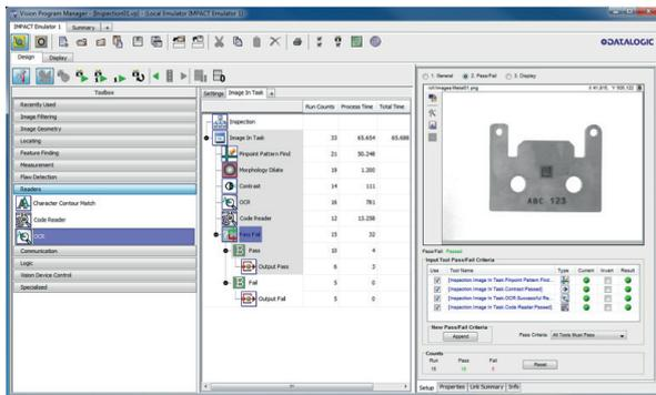
Example of a software platform for Graphical Programming with implemented algorithm for geometric measurement, text and 2D code recognition
