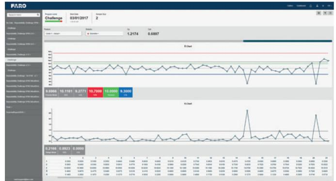
The Repeat Part Management (RPM) Control Center addresses the increasing needs for SPC (Statistical Process Control).
