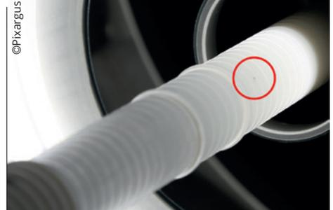
Even flaws too tiny for the human eye to discern are recognized by Profilcontrol 7 S Corrugated Tube in a matter of seconds: holes, dents, blisters, nodes, scratches, fissures, for example, or poorly crimped joints are detected with 100 percent reliability.
