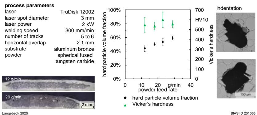
**Fig. 1** Cross section of MMC layers with different powder feed rates; hard particle volume fraction and Vicker's hardness with respect to powder feed rate; indentation of Vicker's hardness measurements in MMC surface
