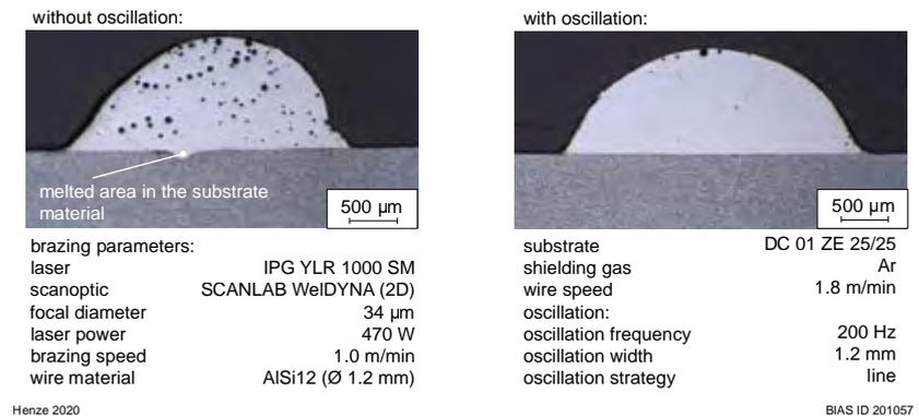
**Fig. 1** Microsections of bead-on-plate seams brazed with keyhole formation without oscillation (left) and with superimposed linear oscillation of the laser beam transverse to the brazing direction.
