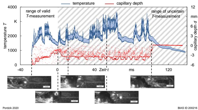
**Fig. 3** Result of the synchronized process observation with measurement of the capillary wall temperature, capillary depth, and high-speed images
