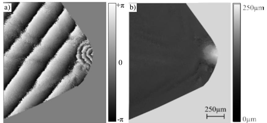
**Fig. 2** Measurement results from the functional surfaces of a carbide insert. Phase values of the measurement showing a significant defect of the functional surface at the tip (right corner; a). Shape data of the carbide insert with the chipping at the tip of the cutting sheath, the chipping has a diameter of about 225  $\mu\text{m}$  and a height difference of more than 200  $\mu\text{m}$ .
