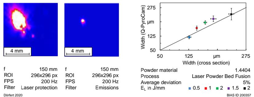
**Fig. 1** (from left to right) Coaxial process monitoring without and with extensive filtering against process emissions as well as the metallographic cross-section of a single track and the measured deviation of the melt pool width between Q-PyroCam images (contains data from [2]).
