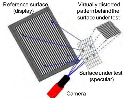
**Fig. 1** Illustration of the principle of Phase Measuring Deflectometry. A camera observes sinusoidal fringe patterns displayed on a monitor in reflection on the surface under test. Displayed patterns are distorted due to the slope of the specular surface. Figure from [4].
