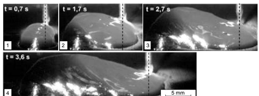
**Fig. 2** Temperature field measurement using a high-speed camera and determination of the melt pool size
