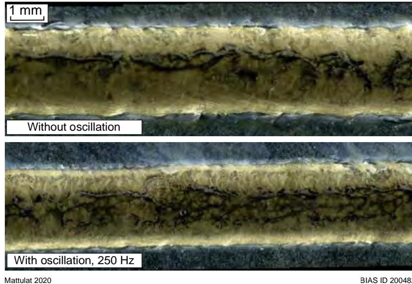
**Fig. 2** Seam edge comparison of laser brazed seams on hot dip galvanized material with and without wire oscillation.
