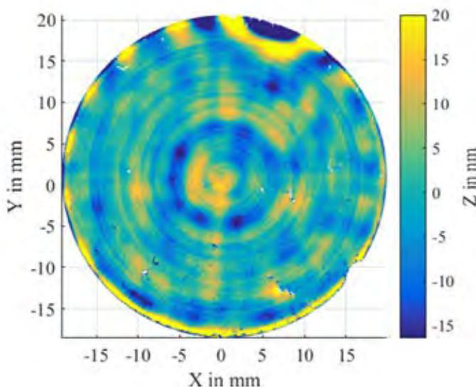
**Fig. 2** Microstructure of a plane mirror manufactured with diamond turning. Measured with PMD. Figure from [1].
