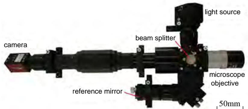
**Fig. 1** Photograph of the digital holographic microscope with the essential optical components.
