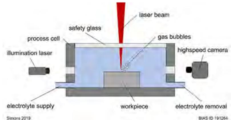
Fig. 1 Schematic representation of the laser chemical test setup
