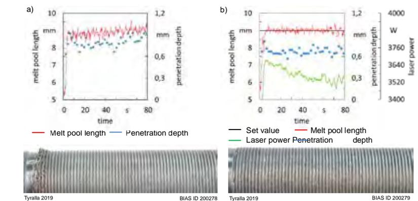
**Fig. 1** Comparison of laser cladding process with online-monitoring (a) and closed-loop control system (b). In the first case, the process applies a laser power of 3.5 kW, whereas the power is adjusted to maintain a constant melt pool length in the controlled case.
