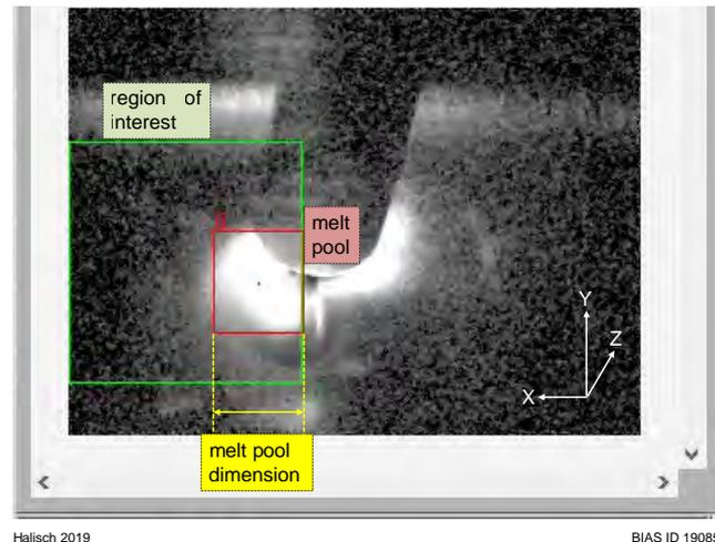
**Fig. 1** Temperature field measurement using Pyrocam and determination of the melt pool size
