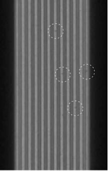
The contrasts of CT images of the internals of batteries are very low, making it difficult to interpret any defects. Artificial intelligence methods such as deep learning provide clarity.
