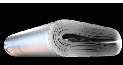
Delaminations, the detachment of the electrode windings or coatings, can be easily visualized with CT.
