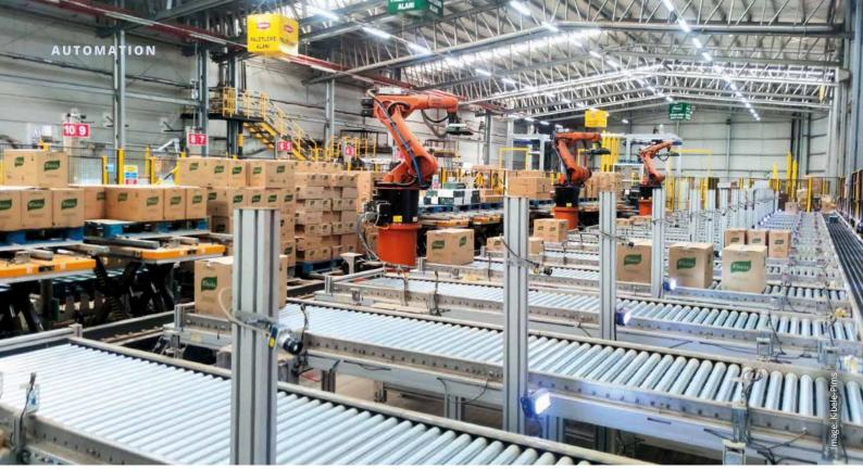
19 cameras enable Knorr food in small boxes to be identified, sorted on 17 lines and prepared for transport on single-type pallets by three robots.
