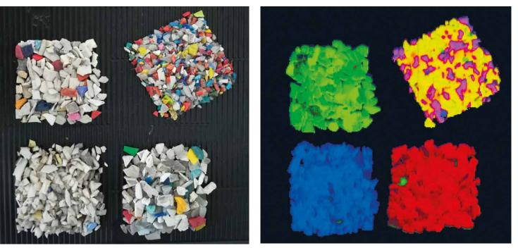
In the image on the right, the different plastics can be easily distinguished by their color as a hyperspectral image: ABS in red, POM in blue, PC in green, PE in yellow and PS in purple.
