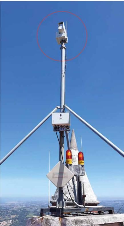
Three industrial cameras from Baumer are concealed in a pan and tilt head. A 360-degree detection requires between four to six minutes in the daytime and approximately 12 minutes at night.
