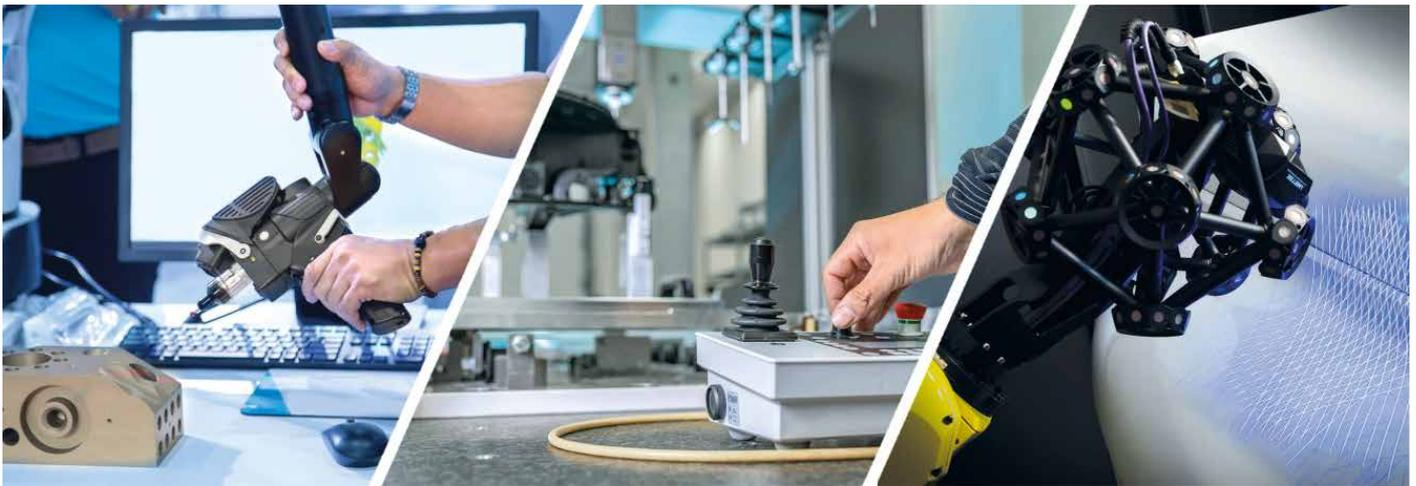
Fig. 4: CMM types: articulated measuring arms – traditional CMMs – robot-guided 3D CMM scanners
