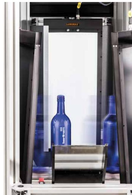
With the collimated Area Lighting solutions from Lumimax, edges and production defects are shown clearly on the object image.
