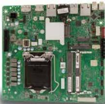
and 35-Watt Thermal Design Power and processors with 8 cores and 65-Watt Thermal Design Power. The two DDR4 SO-DIMM sockets can be equipped with up to 64GB non-ECC memory with a maximum clock frequency of up to 2933 MHz. The integrated graphics unit offers triple display support with a maximum resolution of 4K. An HDMI
