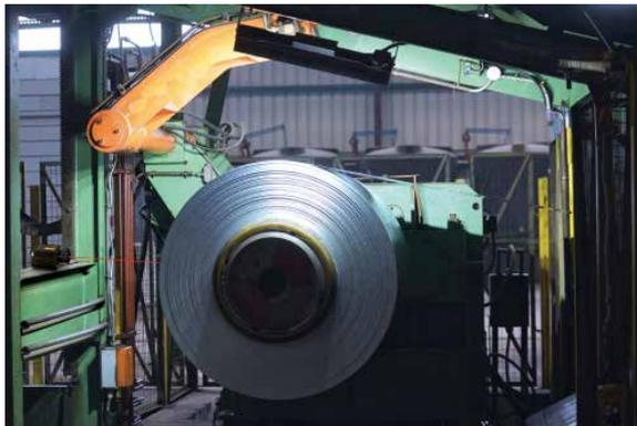
Continuous detection of the coil diameter is necessary in order to monitor the uncoiling process precisely and to determine the changeover time of the coil at an early stage. OptoNCDT ILR2250-100 laser distance sensors from Micro-Epsilon perform this task.
