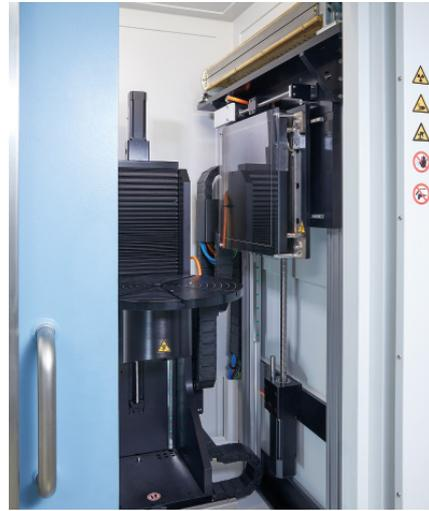
Configuration with flat-panel and line detector
