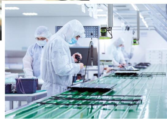
Code readers, which are permanently mounted above control stations, allow a reliable code check on components in order to ensure correct assembly.
