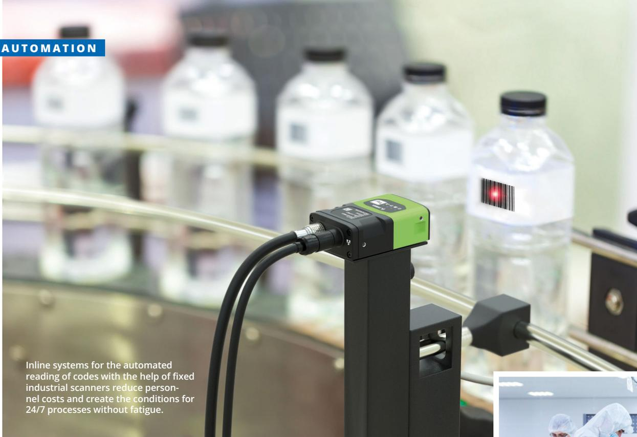
Inline systems for the automated reading of codes with the help of fixed industrial scanners reduce personnel costs and create the conditions for 24/7 processes without fatigue.
