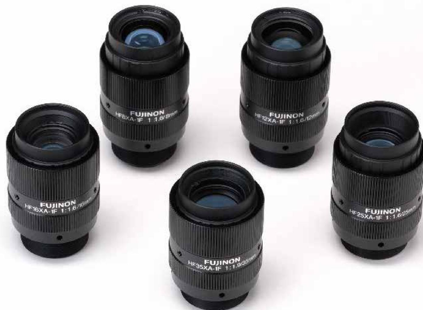
Fujifilm presents the [Fujinon HF-XA-1F series](#) for demanding applications. The series features Fujifilm's Anti Shock & Vibration technology and has a rugged mechanical design with no moving parts inside the lens. The focus is adjusted with the special C-mount and its nut and counter nut system. Users can adapt the iris to their needs by exchanging the screw-locked iris plate. This ensures the highest possible optical stability and durability, even under harsh conditions.
