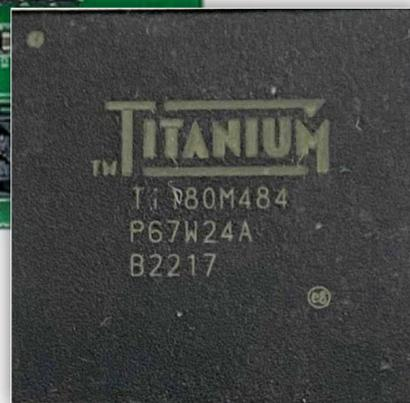
▲ The Titanium Ti180 FPGA is the latest member of the Titanium family and is fabricated in the same 16 nm process node.
