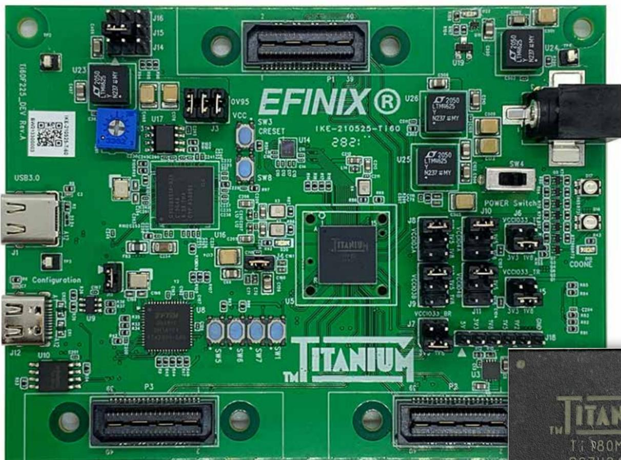
▲ The Titanium Ti60 F225 Development Kit provides a Raspberry Pi camera module and the Ti60 FPGA.
