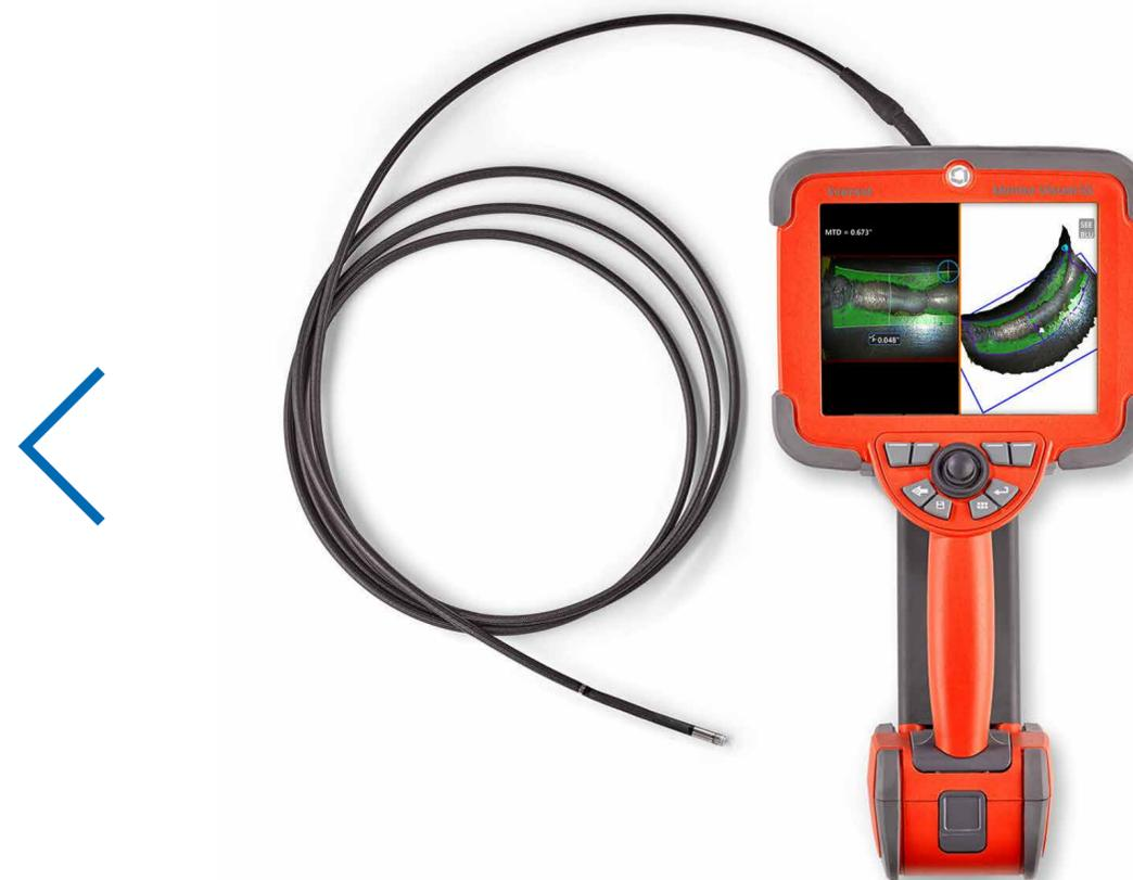
The video borescope Everest Mentor Visual iQ is Suitable for use in all industrial environments. It features a HD camera head combined with built-in connectivity options for better detection and shared decision making without delay.
