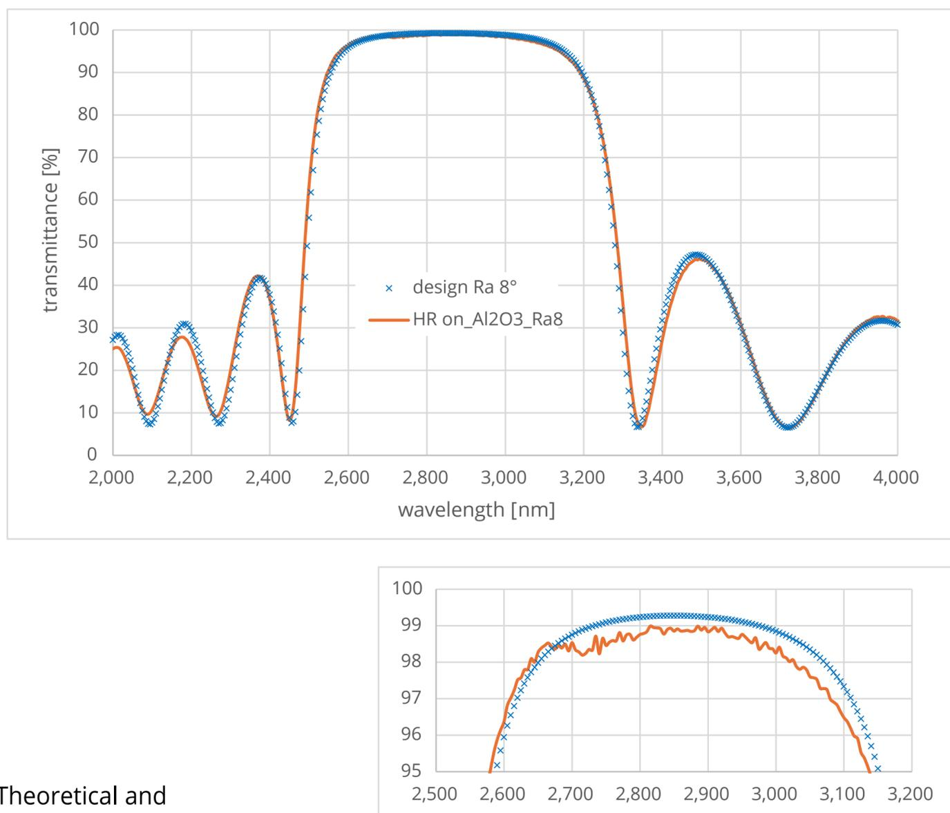
Fig. 5 Theoretical and measured spectra of HR coating on sapphire substrate
