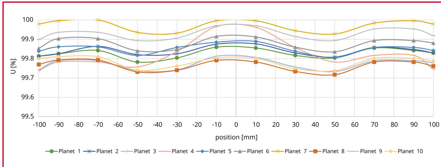
Fig. 3 Nonuniformity of short-wave bandpass filter across ten planets of the double-rotation planetary system
