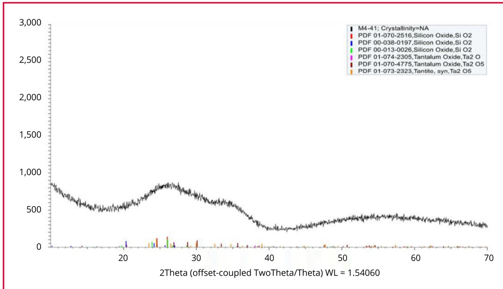
Fig. 4 XRD spectrum of the HR coating based on Ta<sub>2</sub>O<sub>5</sub> / SiO<sub>2</sub> materials
