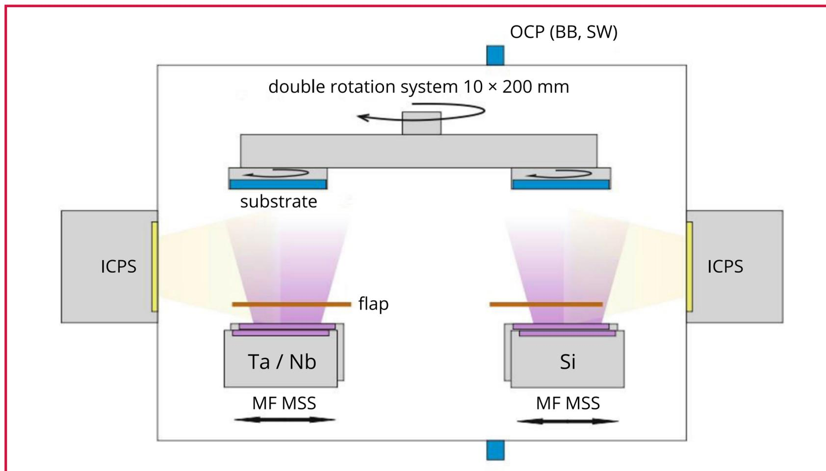
Fig. 1 Scheme of PARMS coating machine Meridian
