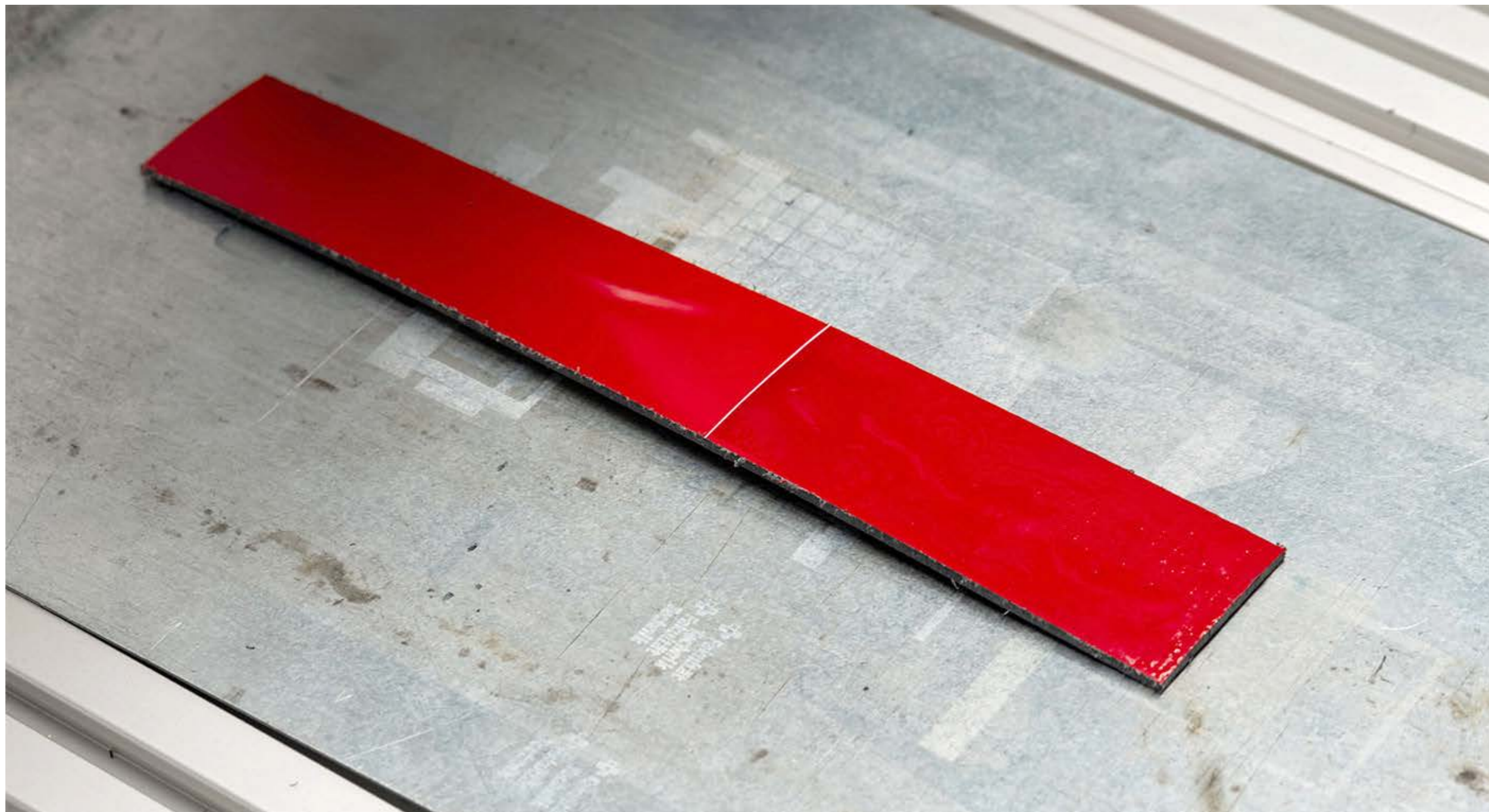
Fig. 2 A simple but ingenious process: the paint is separated from the substrate by laser, whereby a slight color change (right) becomes visible
