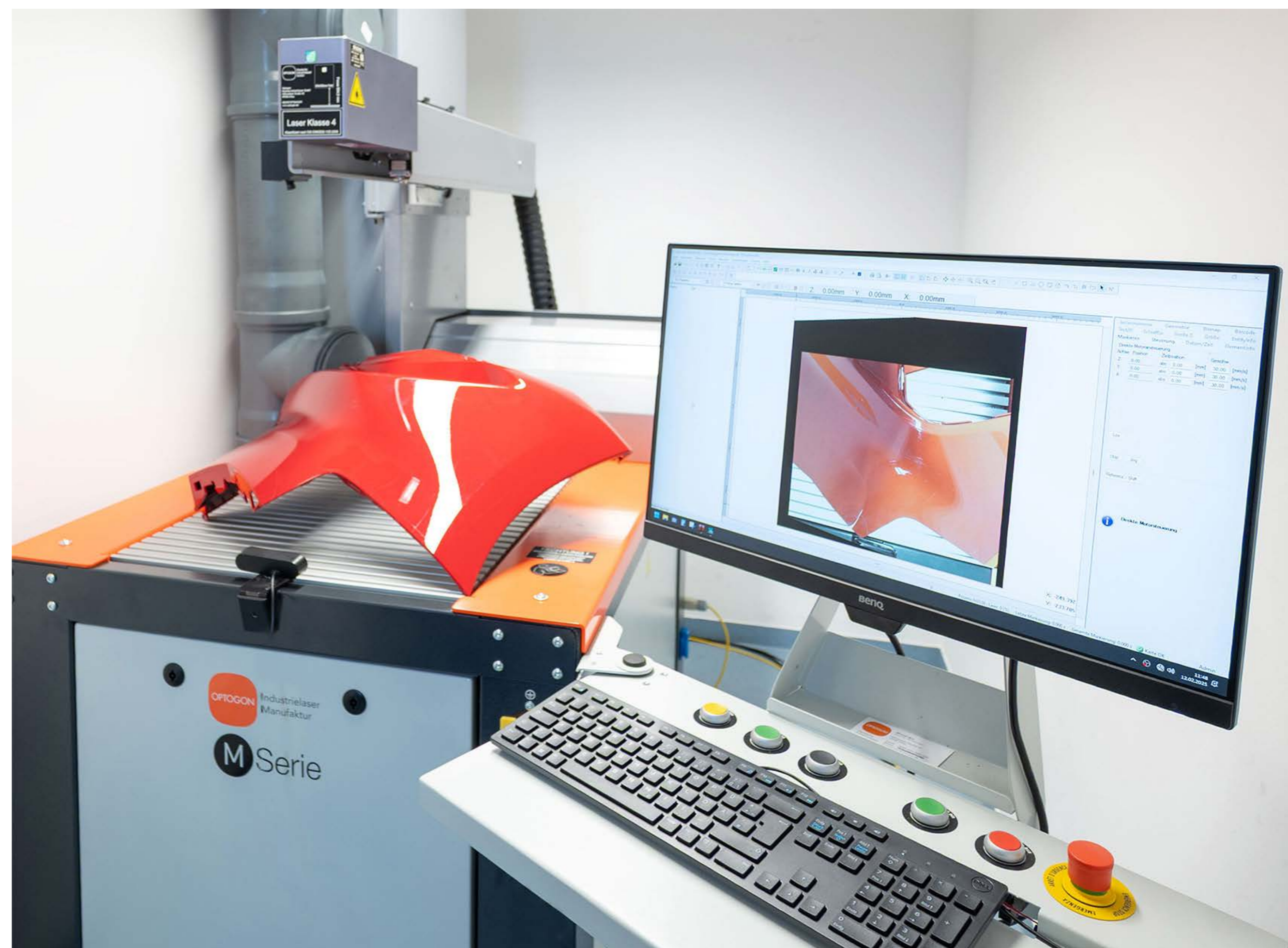
Fig. 1 The computer screen shows a live camera preview of the hybrid component directly at the Optogon M Serie laser: precise and large-area laser decoating using automatic focus interpolation
