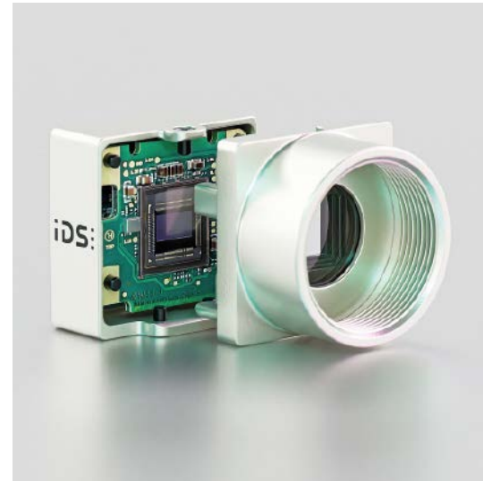
The Ueye XCP-E camera from IDS is a small, lightweight industrial camera with an event-based sensor in a robust die-cast zinc housing (29 × 29 × 17 mm) with screw-on USB Micro-B connection.
