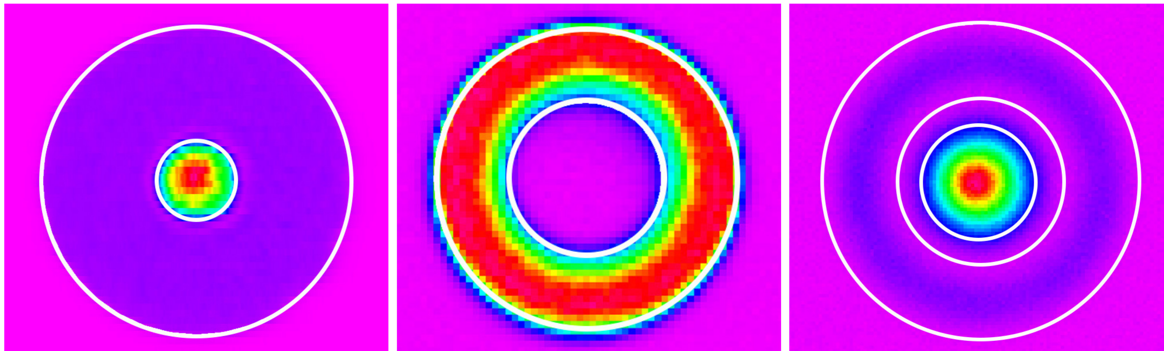
Plateau beam, Donut beam and single mode ring beam evaluated according to the new set of ring beam parameters. The white circles show the diameter of ring and core. These new parameters reflect the characteristics of the beam.
