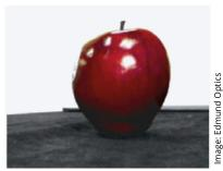
Visible imaging of red apple. Notice the apple looks perfectly red with visible imaging. Defects are not easily discernable.
