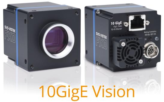
The FXO camera series from SVS-Vistek is based on the latest Sony sensors and provides a 10GigE interface and a C-mount lens connection.
