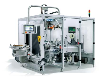
The Caseteq case packer from Christ is a fully automatic horizontal system for erecting, packing and closing pre-glued shipping cases. Cameras from B&R will now be performing various inspection tasks.
