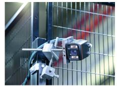
The 3D sensor simultaneously monitors several positions.
