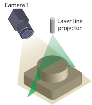
figure 4: Example of laser line scanner. Depth data is calculated by the amount of laser line distortion viewed by the camera.
