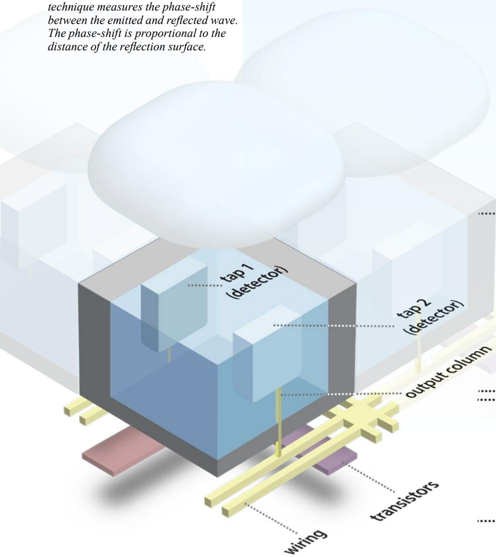
figure 10a: Sony's Current Assisted Photonics Demodulation (CAPD) pixel. Capable of high-speed modulation using drift current in the pixel, allowing for improved accuracy of distance measurement.
