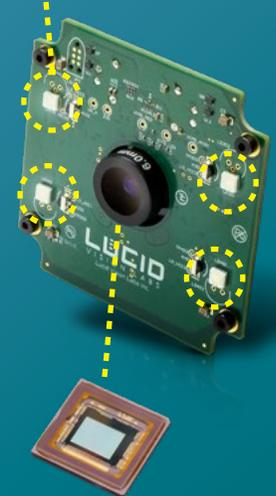
Sony DepthSense IMX556PLR CMOS with 6mm lens
