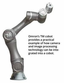
An integrated vision system can improve reliability, consistency and precision. Another advantage is its flexible scalability, based on the needs of the user. For example, it's possible to start with a simple integrated system and then expand it as required. Smart systems based on artificial intelligence (AI) or machine learning (ML) can also help to enhance decision-making through the use of data visualization.
